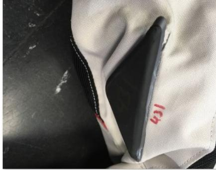
Photo 6: Adhesion carried out with Loctite 431
